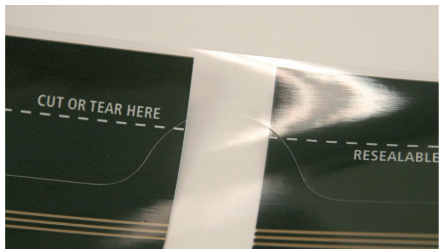
FIGURE 1: Perforating thin films is one of the key processes in food packaging that utilize compact CO 2 lasers.
